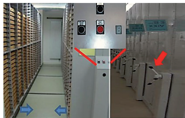
Figure 42. Electronic mobile shelves in Senckenberg DEI, Müncheberg with switch inset (left) and manually operated mobile shelves in the Regional museum in Liberec/CZ (right). Photo credit: Willi Xylander, SMNG.
